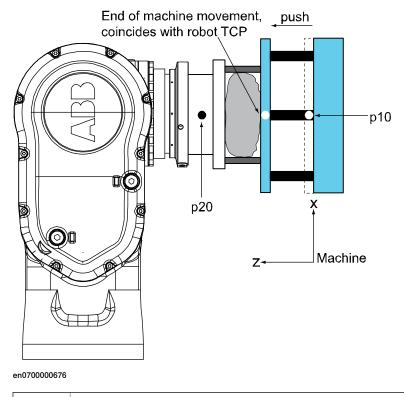
push The external machine pushes the robot away from the position p10.
